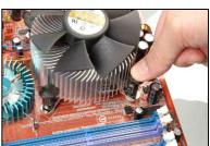
Attach the four-pin power plug from the heatsink and fan assembly to the CPU FAN connector.
